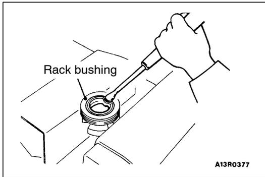
2. Partially bend the oil seal to remove from the rack bushing.
