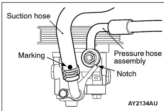
**▶B◀ PRESSURE HOSE ASSEMBLY/SUCTION HOSE INSTALLATION**
