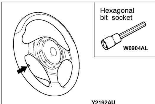
2. Loosen the bolt completely. Then, remove the steering wheel and airbag module assembly.
