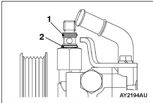
**INSTALLATION SERVICE POINTS****▶A◀ O RING INSTALLATION**
