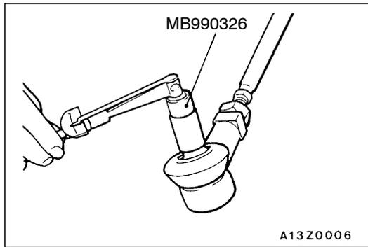
2. Move ball joint stud several times and install nut on stud. Measure ball joint turning torque with special tool.
