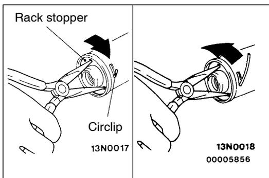
**◀E▶ CIRCLIP REMOVAL**
