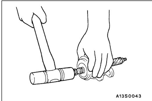
**◀B▶ LOWER OIL SEAL/PINION AND VALVE ASSEMBLY REMOVAL**
