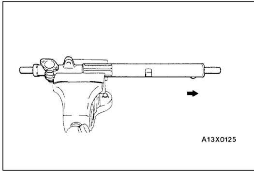
◀F▶ RACK STOPPER/RACK BUSHING/OIL SEAL/O-RING/RACK ASSEMBLY REMOVAL
