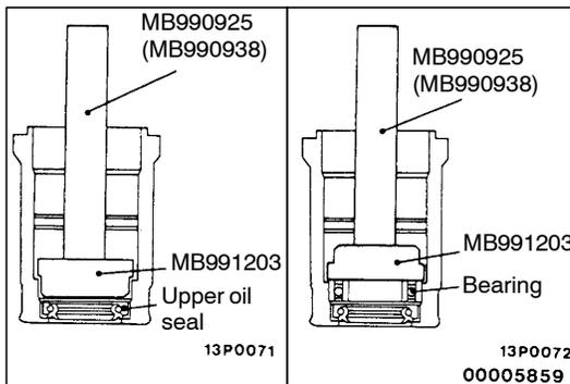
►F◄ UPPER OIL SEAL/UPPER BEARING INSTALLATION
