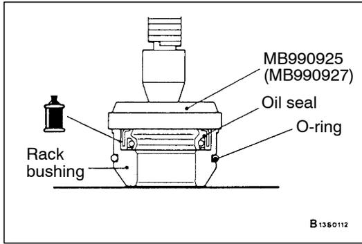
►D◄ OIL SEAL/RACK BUSHING INSTALLATION
