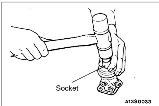
**◀D▶ UPPER BEARING/UPPER OIL SEAL REMOVAL**
