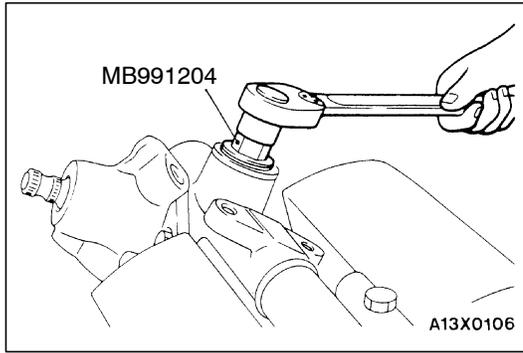
**DISASSEMBLY SERVICE POINTS****◀A▶ RACK SUPPORT COVER REMOVAL**
