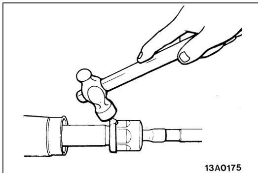
**►L◄ TAB WASHER/TIE ROD INSTALLATION**
