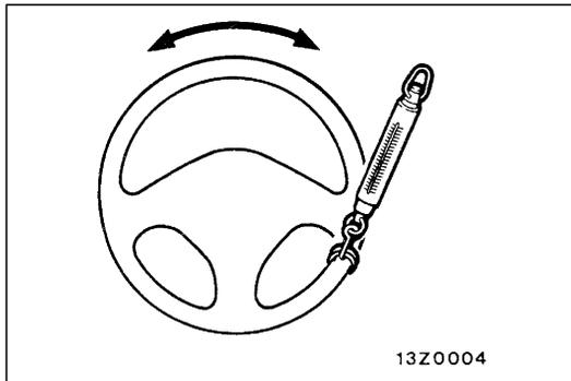
3. When play exceeds the limit, check for play on steering shaft connection and steering linkage. Correct or replace.
