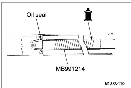
2. Cover the serrations of the rack assembly with the special tool.
