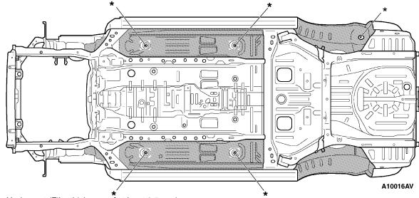
: Undercoat (Film thickness of at least 0.5 mm)
