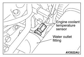
4. Disconnect the engine coolant temperature sensor connector.
