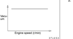
2. Start the engine and check vacuum remains fairly constant after racing the engine.
