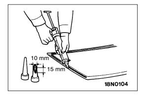
7. Within thirty minutes after the primer application, fill a sealant gun with the adhesive, and then apply the adhesive evenly around the windshield.
