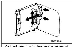
Adjustment of clearance around fuel filler door
