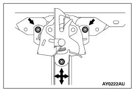
ADJUSTMENT OF ALIGNMENT OF HOOD STEPPED PORTION AND HOOD STRIKER
