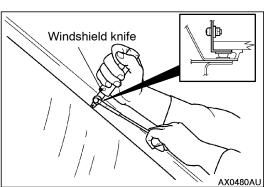
(2) Align the windshield knife blade with the windshield surface and the windshield edge while maintaining an angle of 90 degrees between the windshield knife blade and the windshield edge, and then cut off adhesive by knifing parallel with the windshield edge.
