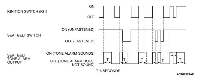
When the ignition switch is turned to ON position without fastening the driver's seat belt (driver's seat belt switch off), the tone alarm will sound for approximately six seconds to warn the driver to fasten the seat belt. When the driver's seat belt is fastened or the ignition switch is turned to OFF position, the tone alarm will stop sounding.
