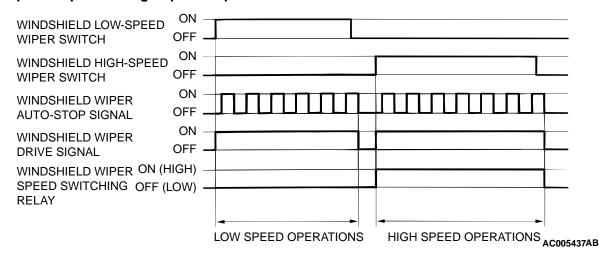
When the ignition switch is at the ACC or ON position, if the windshield low speed wiper switch of the column switch is turned ON, the front-ECU turns ON the windshield wiper drive signal, turns OFF (LO) the windshield wiper speed relay, and operates the wind-
