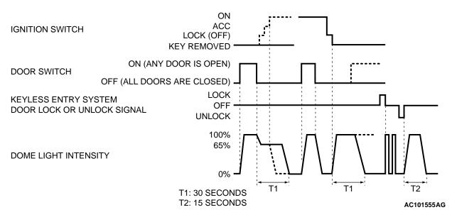
NOTE: The dotted lines in the graph indicate that lighting mode when the ignition switch is turned ON, door is locked, or any door is opened during the timer illumination time.
