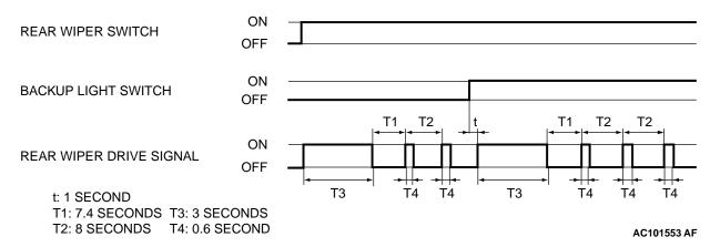
If the rear wiper switch of the column switch assembly is turned ON with the ignition switch in the ACC or ON position, the ETACS-ECU will turn the rear wiper drive signal ON for three seconds (approximately two operations), and then will carry out intermittent operation in a 7.4 to 8-second cycle.
