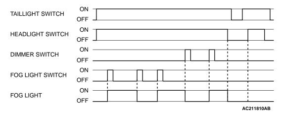
The fog lights will illuminate only when the fog light switch is operated while the low-beam headlights are on.
