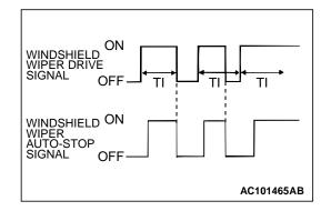
The front-ECU determines the intermittent time TI from the input SWS data signal, and turns ON the windshield wiper drive signal. When the wiper is at the STOP position, the windshield wiper auto-stop signal goes OFF to turn OFF the windshield wipe drive signal. After the intermittent time TI seconds from when the windshield wiper drive signal turned ON, the windshield wiper drive signal is turned ON again and the above operation is repeated.
