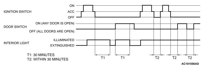
Illuminated interior lights such as the front dome light, etc. (all lights using the dome light fuse as the power supply) will automatically go off in the following conditions to prevent the battery from discharging as a result of forgetting to turn off the lights or incomplete closing of the door.
