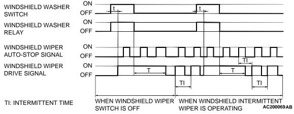
When the ignition switch is at the ACC or ON position, if the windshield washer switch of the column switch is turned ON, the front-ECU turns ON the windshield washer relay. The windshield wiper drive signal is turned ON in 0.3 seconds until three seconds after the windshield washer switch goes OFF to
