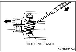
2. Insert the tip of a screwdriver [0.8 mm (0.03 inch) width] into the connector as shown in the figure, push it lightly to raise the housing lance, and pull out the terminal.
