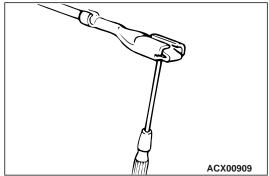
3. Insert a screwdriver through the hole provided on the terminal and raise the contact point. Lightly squeeze the outer edge so the flats are parallel with the bottom.
