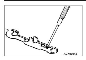
3. Press the contact point of the female terminal down by holding a screwdriver [1.4 mm (0.06 inch) width] as shown in the figure. Lightly squeeze the outer edge so the flats are parallel with the bottom.
