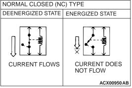
Relays may be classified as the normally open-type or the normally closed-type, depending on their contact construction.
