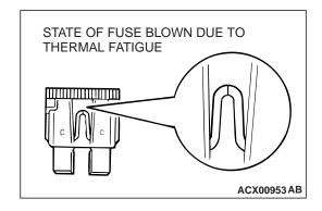
2. Fuse blown due to repeated turning current on and off
