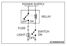
2. By using a relay, a heavy current can be turned on and off by a switch using much less current. For example, in the circuit shown here, when the switch is turned on (closed), current flows to the coil of the relay. Then, its contact is turned on (closed) and the light comes on. The current flowing through the switch is much less than that for the light.
