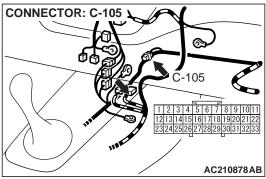
Q: Are the harness wires between joint connector (6) C-105 terminal 28 and fan control relay connector A-09X terminal 1 damaged?
