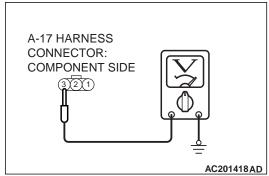
STEP 2. Check the fan control relay.
