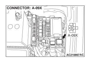
STEP 6. Check for harness damage between fan control relay connector A-09X terminal 3 and ground.
