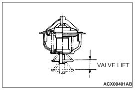
2. Check that the amount of valve lift is at the standard value when the water is at the full-opening temperature.
