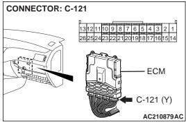
Q: Are the harness wires between ECM connector C-121 terminal 21 and fan control module connector A-17 terminal 2 damaged?
