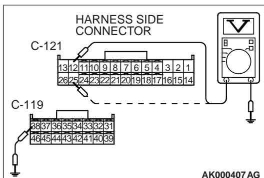
**STEP 9. Measure the power supply voltage at ECM harness side connector C-121, C-119.**
