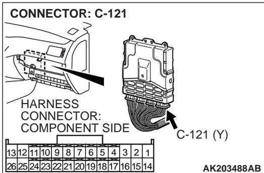
**STEP 10. Check connector C-121 at ECM for damage.**
