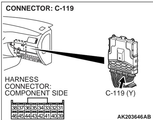
**STEP 6. Measure the power supply voltage ECM connector C-119.**
