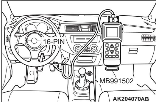
**STEP 3. Using scan tool MB991502 or MB991958, check data list.**
