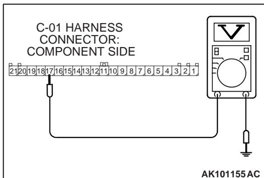
**STEP 2. Check for continuity at combination meter harness side connector C-01.**
