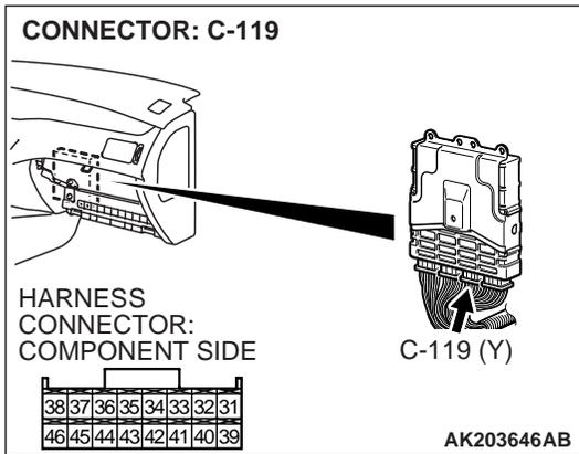
**STEP 5. Check connector C-119 at ECM for damage.**
