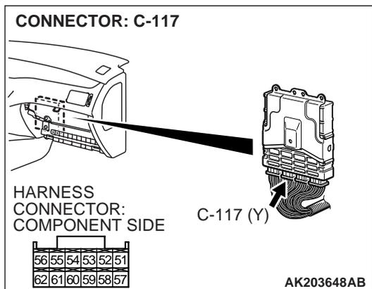
**STEP 2.** Check for open circuit, short circuit to ground and harness damage between data link connector C-14 (terminal No. 7) and ECM connector C-117 (terminal No. 62).
