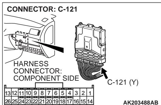
**STEP 9. Check for harness damage between injector connector and ECM connector.**
