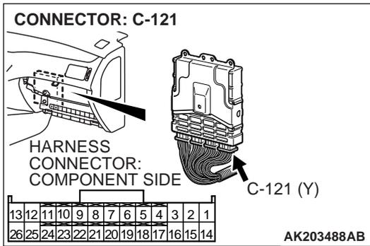
**STEP 9. Check connector C-121 at ECM for damage.**
