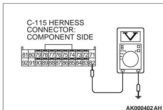
**STEP 5. Measure the ignition switch-IG signal voltage at ECM harness side connector C-115.**
