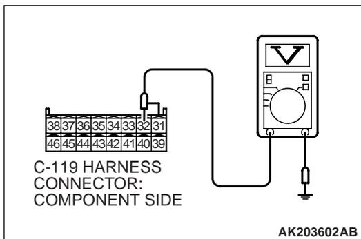
**STEP 3. Measure the output voltage at ECM harness side connector C-119.**
