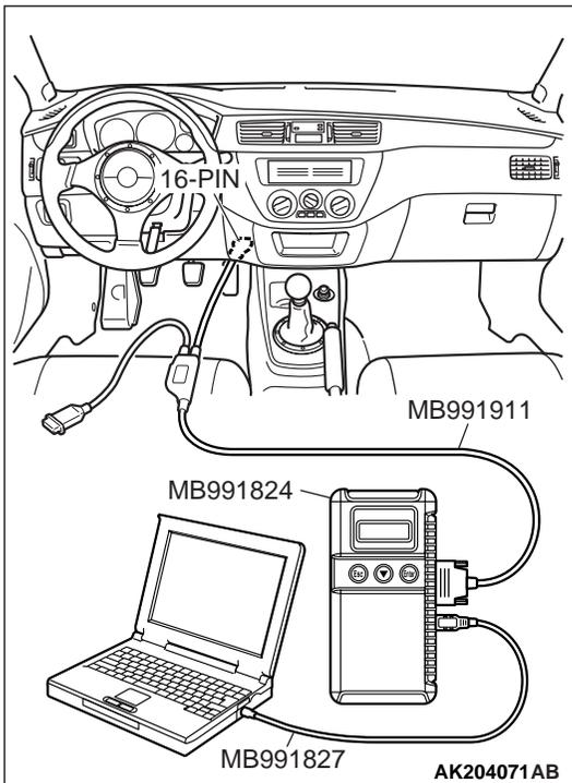
**STEP 1.** Using scan tool MB991502 or MB991958, read the diagnostic trouble code (DTC).
