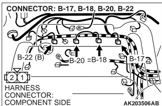
**STEP 6. Check harness connectors B-22 or B-20 or B-18 or B-17 at injector for damage.**
