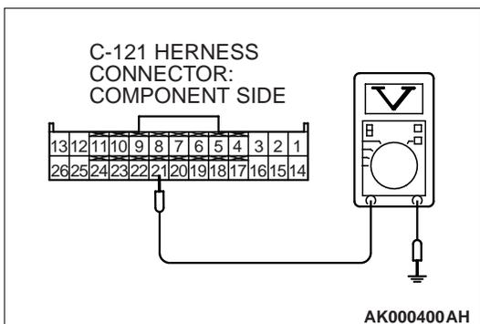
**STEP 2. Check the output voltage at ECM harness side connector C-121.**
