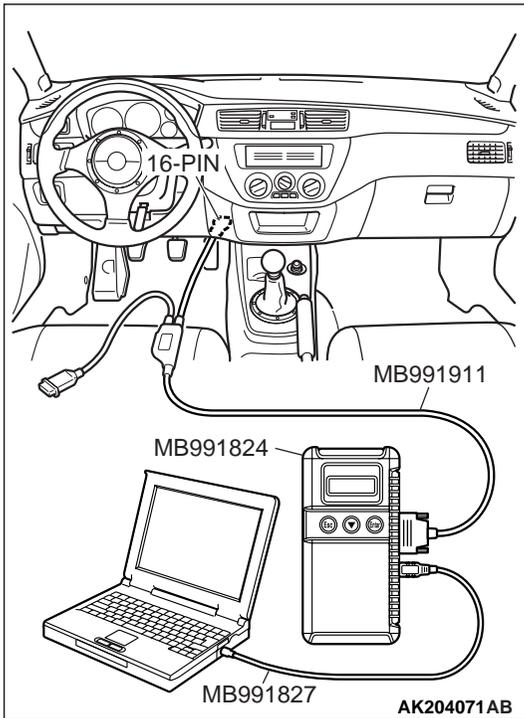
**STEP 10. Using scan tool MB991502 or MB991958, check data list.**
