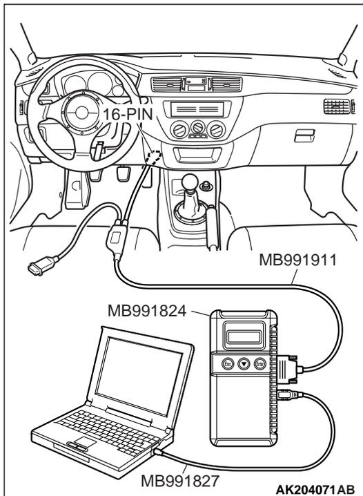
**STEP 6. Using scan tool MB991502 or MB991958, check data list.**
