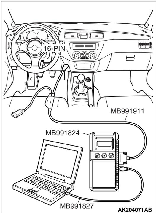
**STEP 7. Using scan tool MB991502 or MB991958, check data list item 11: heated oxygen sensor (front).**
