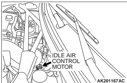
**STEP 2. Check the idle air control (IAC) motor operation sound.**
