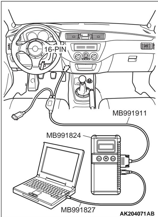
**STEP 5. Using scan tool MB991502 or MB991958, check actuator test.**
