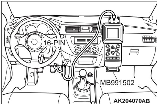
**STEP 9. Using scan tool MB991502 or MB991958, check data list.**
