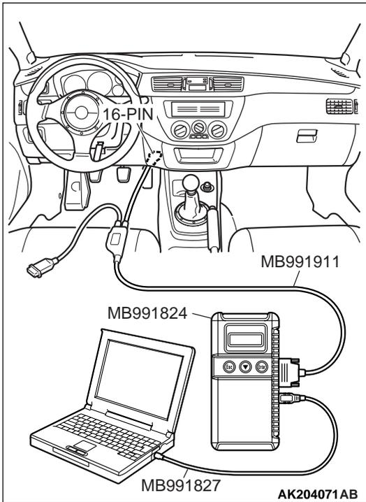
**STEP 7. Using scan tool MB991502 or MB991958, check data list.**
