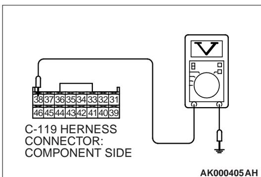
**STEP 8. Measure the power supply voltage at ECM harness side connector C-119.**
