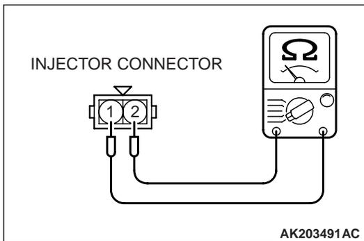
(2) Measure the resistance between each injector side connector terminal No. 1 and No. 2.
