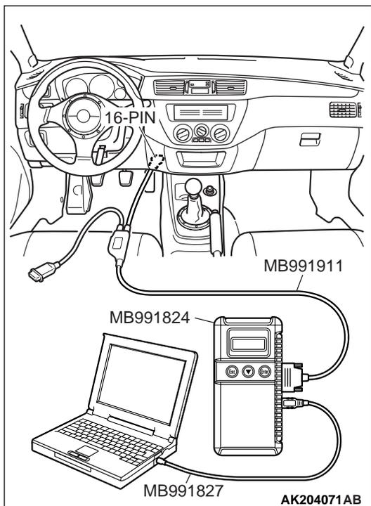
**STEP 5. Using scan tool MB991502 or MB991958, check data list item 45: Idle Air Control Position.**
