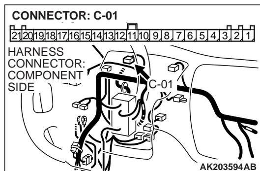
**STEP 4. Measure the power supply voltage at combination meter harness side connector C-01.**
