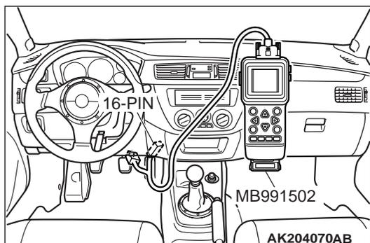
**STEP 4. Using scan tool MB991502 or MB991958, check actuator test.**
