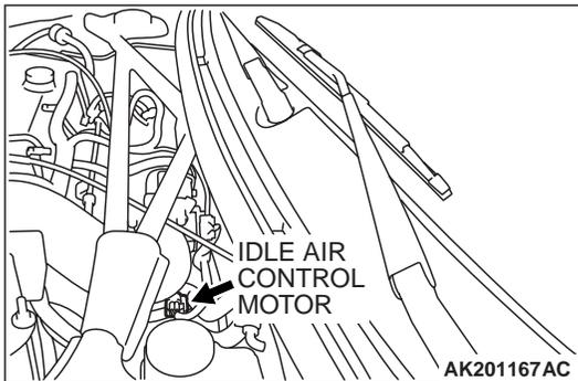
**STEP 6. Check the idle air control (IAC) motor operation sound.**
