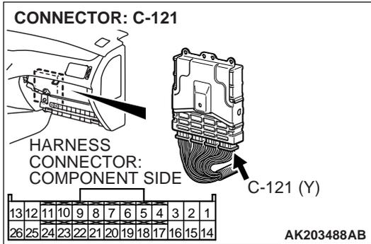
**STEP 2. Measure the output voltage at ECM harness side connector C-121.**
