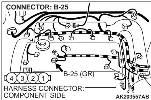
**STEP 3. Check connector B-25 at generator connector for damage.**
