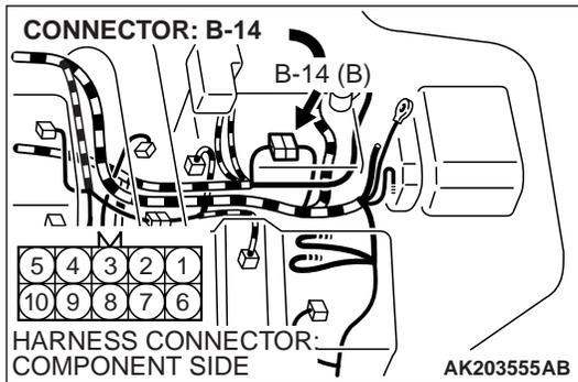
**STEP 2. Check connector B-14 at generator intermediate connector for damage.**
