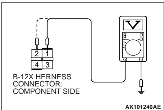
**STEP 3. Measure the power supply voltage at MFI relay harness side connector B-12X.**
