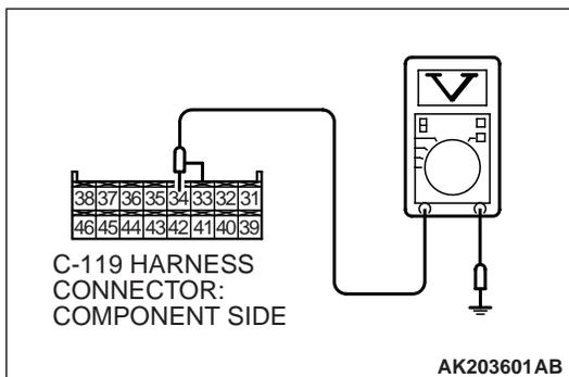
**STEP 2. Measure the output voltage at ECM harness side connector C-119.**
