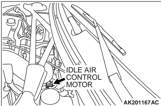
**STEP 5. Check the idle air control (IAC) motor operation sound.**
