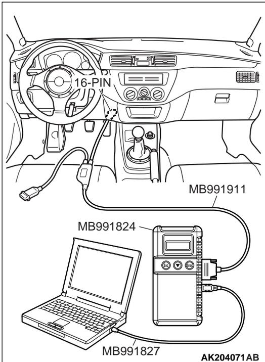
**STEP 4. Using scan tool MB991502 or MB991958, check actuator test.**
