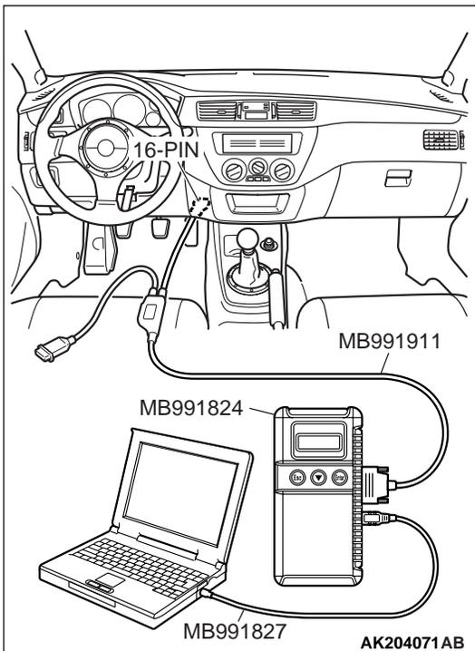
**STEP 2. Using scan tool MB991502 or MB991958, check actuator test items 01, 02, 03, 04: Injector.**
