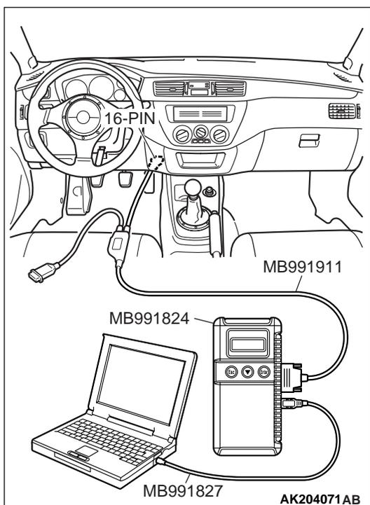
**STEP 8. Using scan tool MB991502 or MB991958, check actuator test.**
