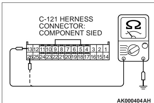
**STEP 7. Check for continuity at ECM harness side connector C-121.**
