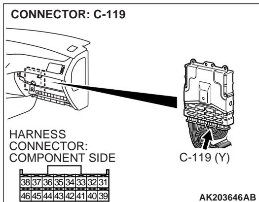
**STEP 4. Check connector C-119 at ECM for damage.**
