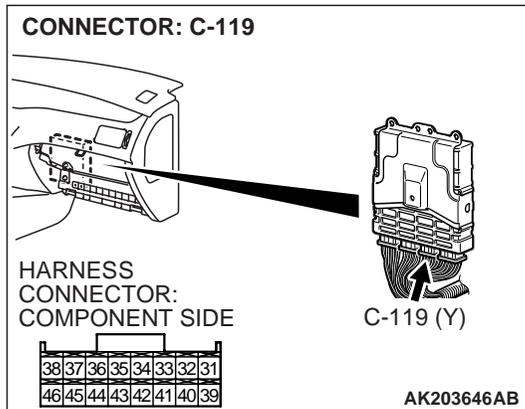
**INSPECTION PROCEDURE 27: INCORRECT IDLE SPEED WHEN THE A/C IS OPERATING (A/C SWITCH 2 SIGNAL)**
