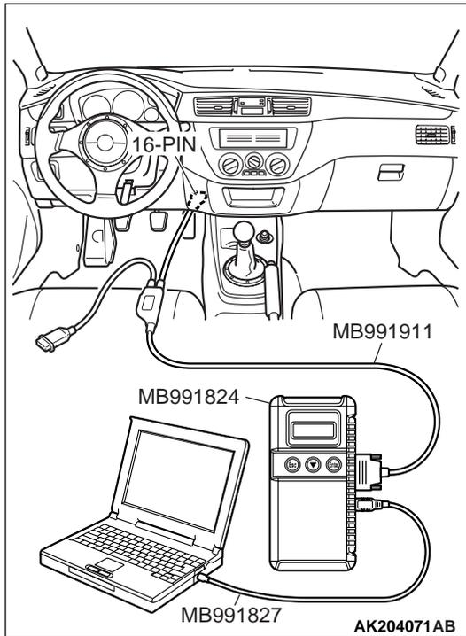
**STEP 2. Using scan tool MB991502 or MB991958, check actuator test.**
