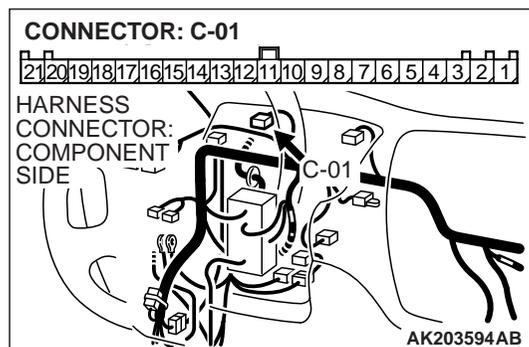
**STEP 3. Check connector C-01 at the combination meter for damage.**
