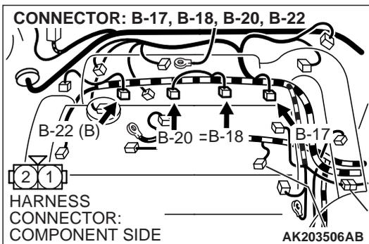
**STEP 10. Check for harness damage between injector connector and ECM connector.**
