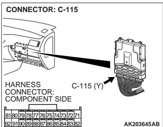
**STEP 4. Check connector C-115 at ECM for damage.**
