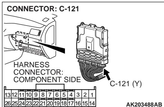
**STEP 11. Check for harness damage between injector connector and ECM connector.**
