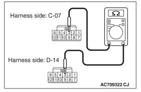
C-07 WCM connector terminal No.3 –D-14 receiver antenna assembly connector terminal No.3.
