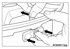
4. While maintaining the TPMS transmitter contact with the rim by applying pressure to the back of the valve, slightly press on the cap to wards the center of the wheel in order to adapt the angle of the valve/TPMS transmitter to the profile of the rim.
