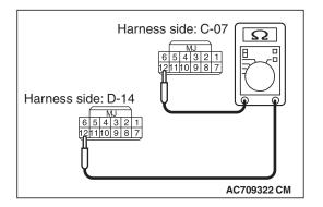
C-07 WCM connector terminal No.12 –D-14 receiver antenna assembly connector terminal No.12.
