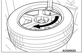
4. Turn the wheel in order to engage all the first side of the tire. NOTE: The standard shoes can pass over the sensor without damaging it.
