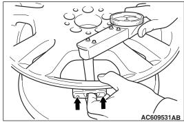
While maintaining the TPMS transmitter and valve in position, screw the nut with a torque wrench.
