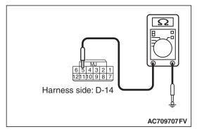
(4) Check the wiring harness between receiver antenna assembly connector D-14 (terminal No.5) and ground
