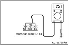
(3) Check the wiring harness between receiver antenna assembly connector D-14 (terminal No.3) and ground
