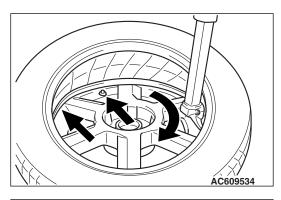
3. Engage the shoe and make sure that 20 cm (7.9 inch) is maintained between the cross point and the valve.
