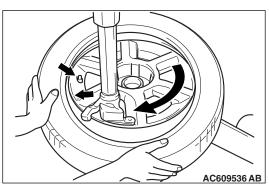
5. Put the second side of the tire in position, so that the cross point of the belt with the rim is approximately 20 cm (7.9 inch) away from the valve. The curved arrow shows the direction of rotation of the wheel.
