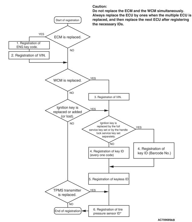
\*: When WCM or TPMS transmitter is replaced.
