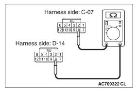
C-07 WCM connector terminal No.8 –D-14 receiver antenna assembly connector terminal No.8.
