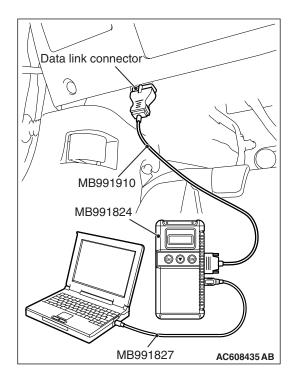
STEP 2. Using scan tool MB991958, read the combination meter diagnostic trouble code.
