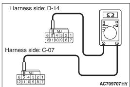
(4) Check the wiring harness between receiver antenna assembly connector D-14 (terminal No.5) and WCM connector C-07 (terminal No.5).
