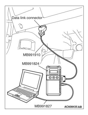
STEP 2. Using scan tool MB991958, check for diagnostic trouble code.
