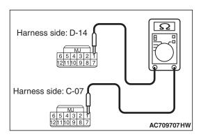
STEP 7. Check the wiring harness between the receiver antenna assembly connector D-14 (terminal Nos. 1, 3 and 5) and the WCM connector C-07 (terminal Nos. 1, 3 and 5) for open circuit.
