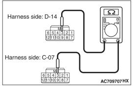
(3) Check the wiring harness between receiver antenna assembly connector D-14 (terminal No.3) and WCM connector C-07 (terminal No.3).
