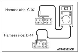
C-07 WCM connector terminal No.5 –D-14 receiver antenna assembly connector terminal No.5.
