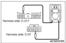
(3) Check the wiring harness between WCM connector C-07 (terminal No.9) and ETACS-ECU connector C-317 (terminal No.5)
