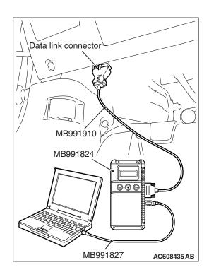
STEP 2. Using scan tool MB991958, read the audio visual navigation unit diagnostic trouble code.
