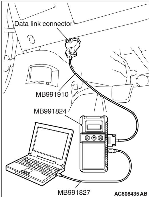
**STEP 1. Check the ETACS-ECU coding data.**
