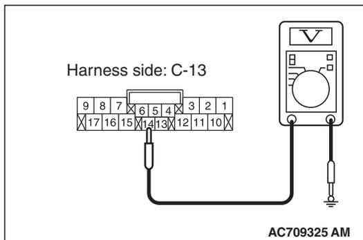
**STEP 11. Check the wiring harness between multivision display connector C-13 (terminal 14) and ETACS-ECU connector C-315 (terminal 9).**
