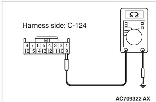
**STEP 3. Check the ground circuit to the center panel unit. Measure the resistance at center panel unit connector C-124.**
