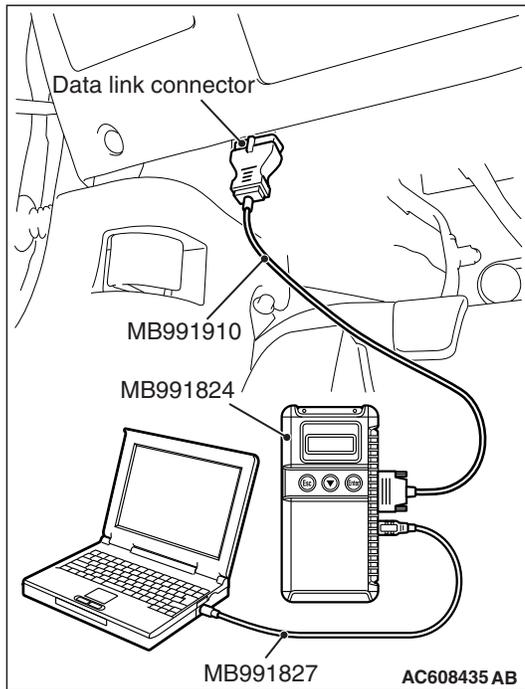
**STEP 1. Using scan tool MB991958, diagnose the CAN bus line.**
