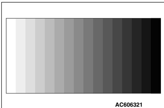
4. When "Enter" is pressed while the gray scale is shown with a 16-step gradation, a crosshatch pattern will be displayed (Each cell should be square).
