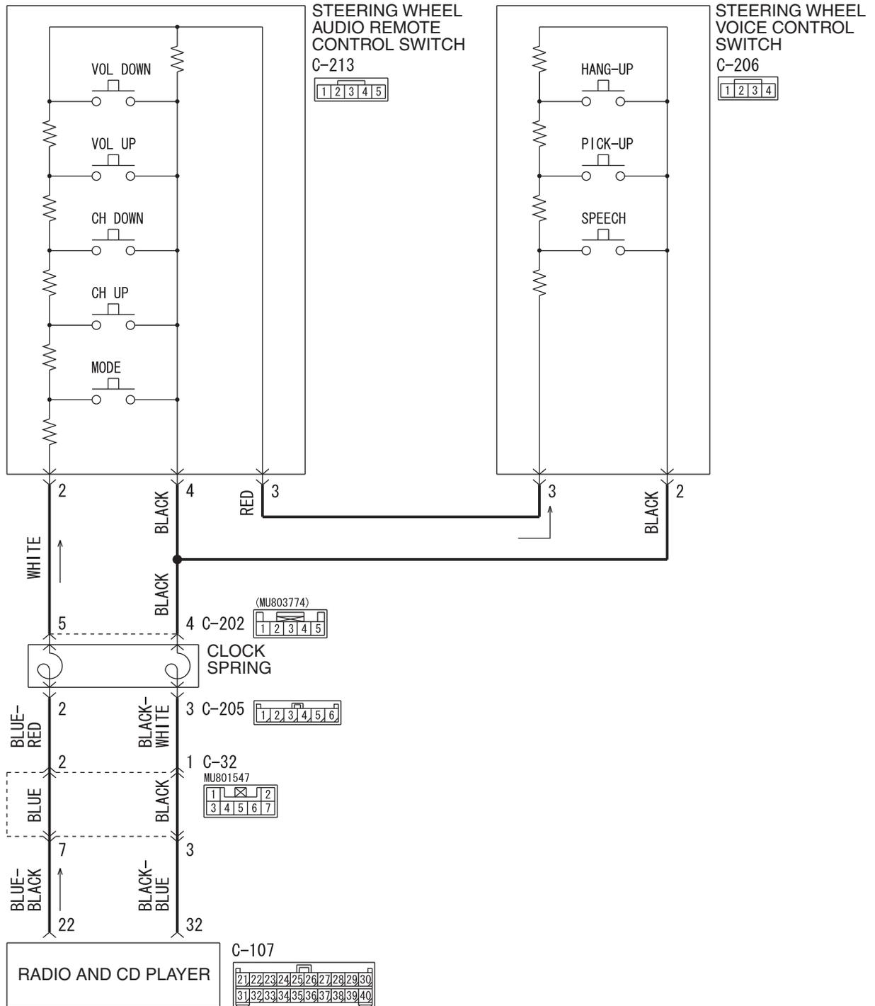
Steering Wheel Voice Control Switch Circuit <Vehicles With MMCS>
