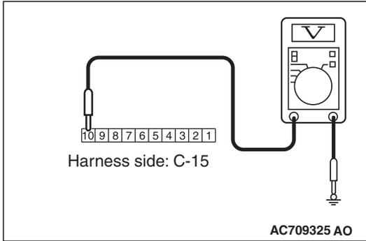
**STEP 8. Check the battery power supply circuit to the CAN box unit. Measure the voltage at CAN box unit connectors C-15.**
