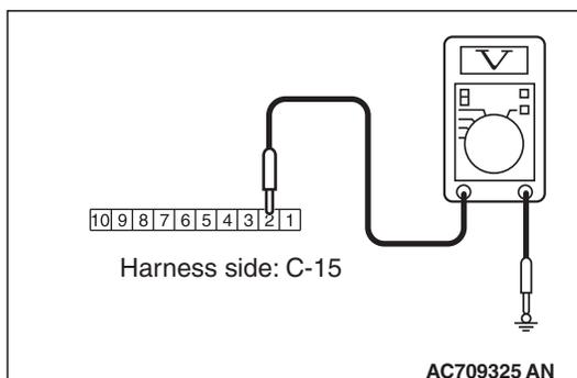
**STEP 5. Check the wiring harness between CAN box unit connector C-15 (terminal 2) and fusible link (36).**
