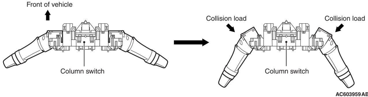
If the column switch is moved to the front of the vehicle and hit on the instrument panel or meter bezel by the frontal collision of vehicle, the steering wheel is moved to the front of the vehicle because the right and left levers fall down, ensuring the driver's safety. In addition, the column switch secures the rigidity that the levers do not fall down by the normal operation, however, it cannot be reused after the deformation.
