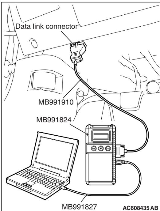
**STEP 2. Using scan tool MB991958, read the SRS-ECU diagnostic trouble code**
