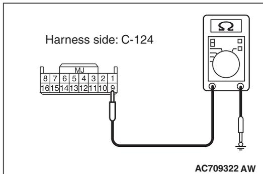
**STEP 5. Check the wiring harness between center panel unit connector C-124 (terminal 9) and ground.**
