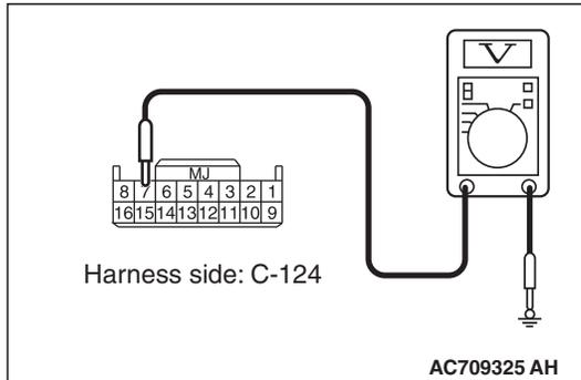
**STEP 6. Check the power supply circuit to the center panel unit. Measure the voltage at center panel unit connector C-124.**
