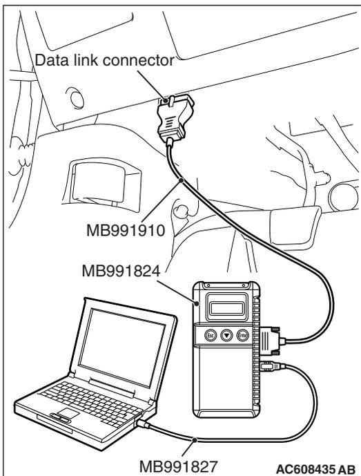
**STEP 3. Check the MMCS service mode, CAN communication confirmation, and coding data.**
