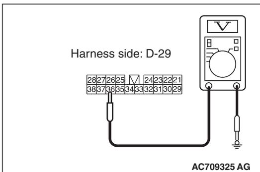
**STEP 11. Check the power supply circuit to the audio amplifier. Measure the voltage at audio amplifier connector D-29.**
