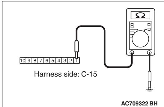
**STEP 2. Check the ground circuit to the CAN box unit.**
