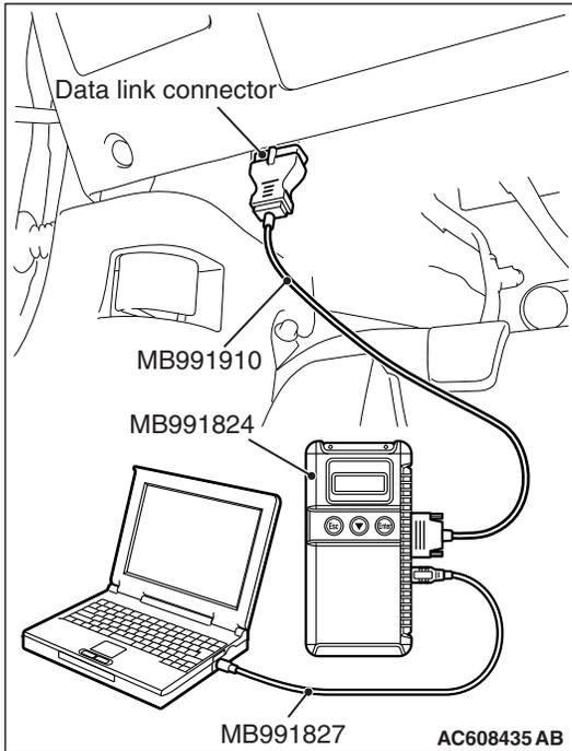
**STEP 2. Using scan tool MB991958, Check whether the diagnostic trouble code is reset.**
