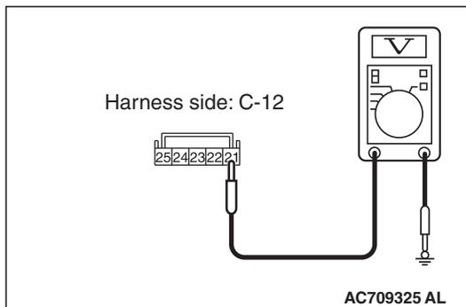
**STEP 6. Check the power supply circuit to the multivision display. Measure the voltage at multivision display connector C-13, C-12.**
