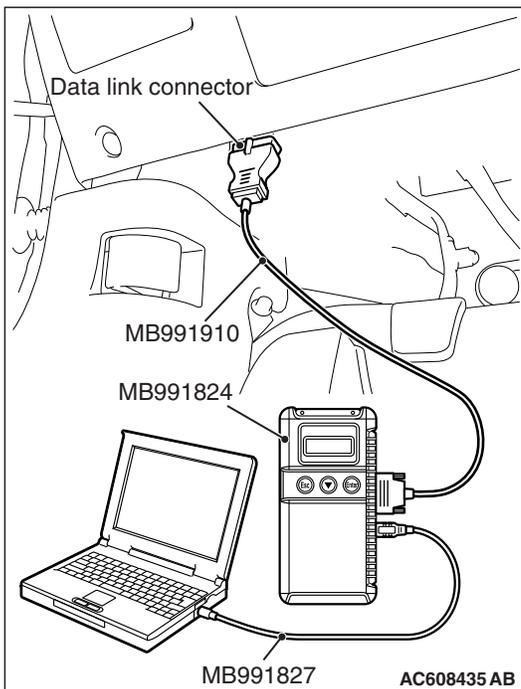
**STEP 2. Using scan tool MB991958, read the ETACS-ECU diagnostic trouble code**
