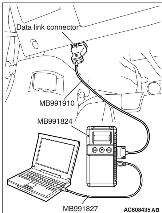
**STEP 1. Using scan tool MB991958, read the diagnostic trouble code.**
