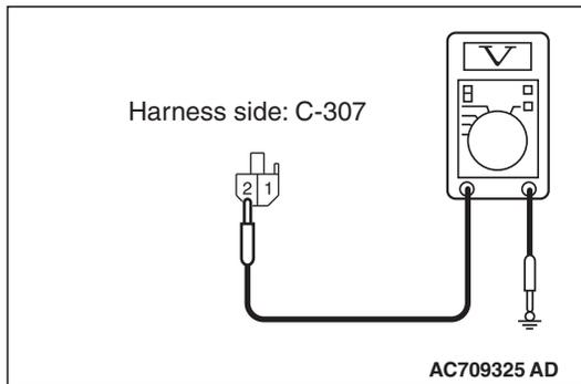
**STEP 8. Check the wiring harness between ETACS-ECU connector C-307 (terminal 2) and fusible link (36)**
