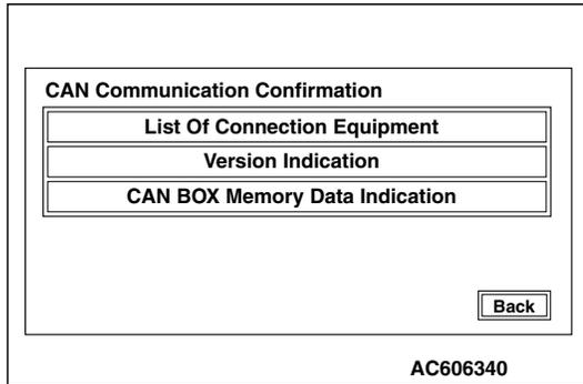
2. If "List Of Connection Equipment" is selected on "CAN Communication Confirmation" screen, the system will determine which equipment is installed according to the connected equipment reference table. Then the equipment which are connected to the CAN box unit will be displayed.
