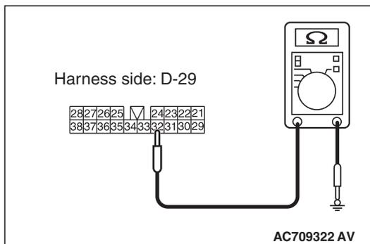
**STEP 13. Check the ground circuit to the audio amplifier. Measure the resistance at audio amplifier connector D-29.**
